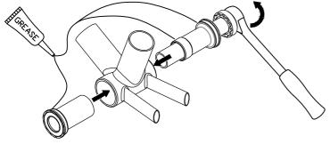
$\begin{array}{l} \textbf{Step 1} \\ \textbf{Apply thin layer of grease to adaptors and threads} \end{array}$
