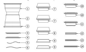
$\widehat{\mbox{(13)}}$  and  $\widehat{\mbox{(14)}}$  are micro adjustment spacers and only need to be used to make small adjustments to the chainline.
