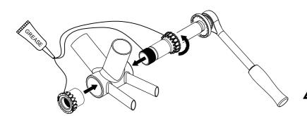
Step 1 Apply thin layer of grease to BB cups as shown in the diagram.
