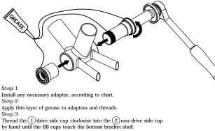
Use a torque wrench with the (3)BB Installation Tool to tighten to 25-30 N.m (221-266 in-lb).
