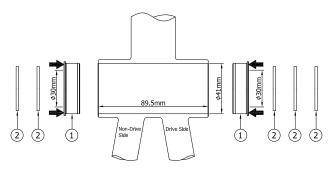
Only apply pressure to flange when installing to prevent bearing damage.
