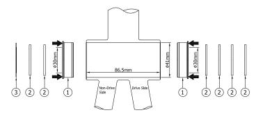
Only apply pressure to flange when installing to prevent bearing damage.
