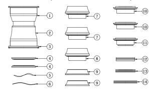
(3) and (4) are micro adjustment spacers and only need to be used to make small adjustments to the chainline.
