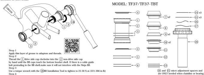
Install any necessary adaptor, according to this manual.
